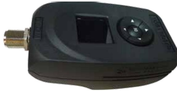
The UglyBox is hailed as the 'riggers best friend', an indispensable tool in the lighting designer or technician's arsenal. With the capability to receive W-DMX™ signals to check their signal strength, as well as check the output of DMX channels, the W-DMX™ UglyBox is great for testing the limits of the W-DMX™ radio system and/or checking DMX data, in a portable, pocket sized device.
