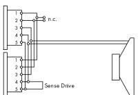
NLT4 F/M/NL4 and EP5 connector wiring
