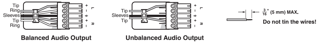
Figure 4. Audio Output Connector Wiring
