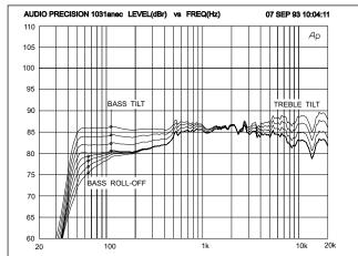
Figure 5. The curves show the effect of the bass tilt, treble tilt and bass roll-off controls on the free field response.
