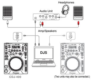
•Configuration when using an External DJ mixer (Example of Connections)
