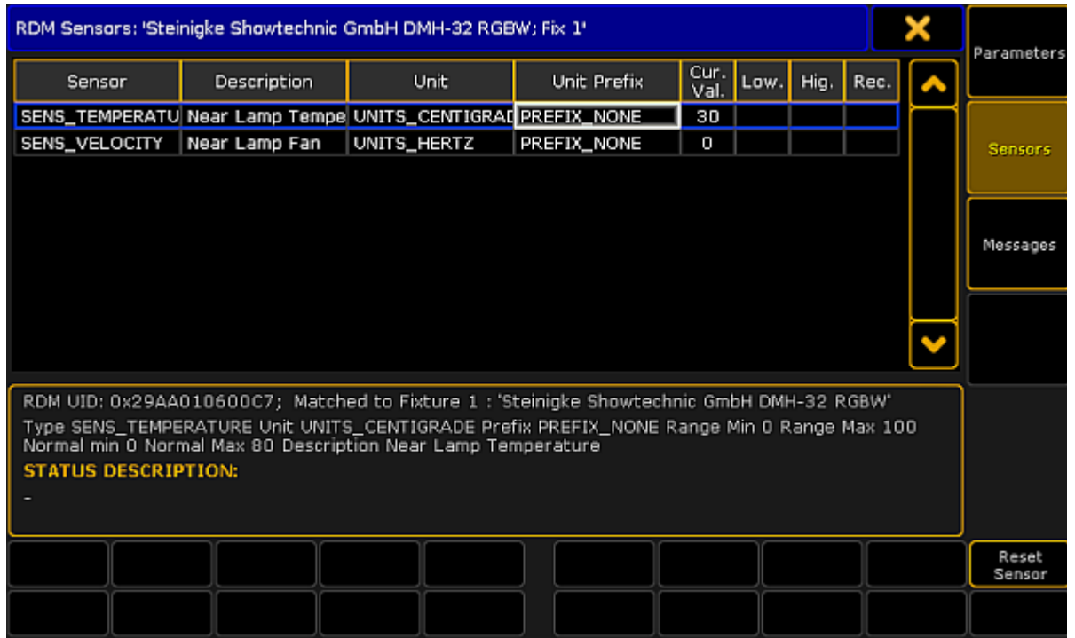
RDM sensors window
