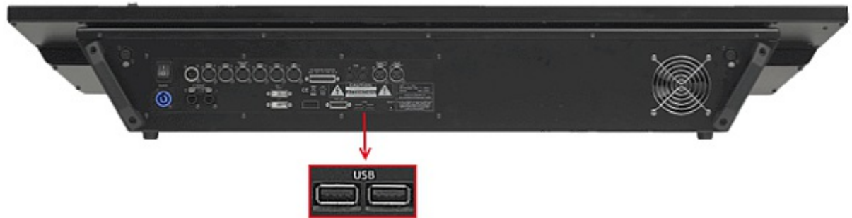
grandMA2 full-size USB connector rear panel
