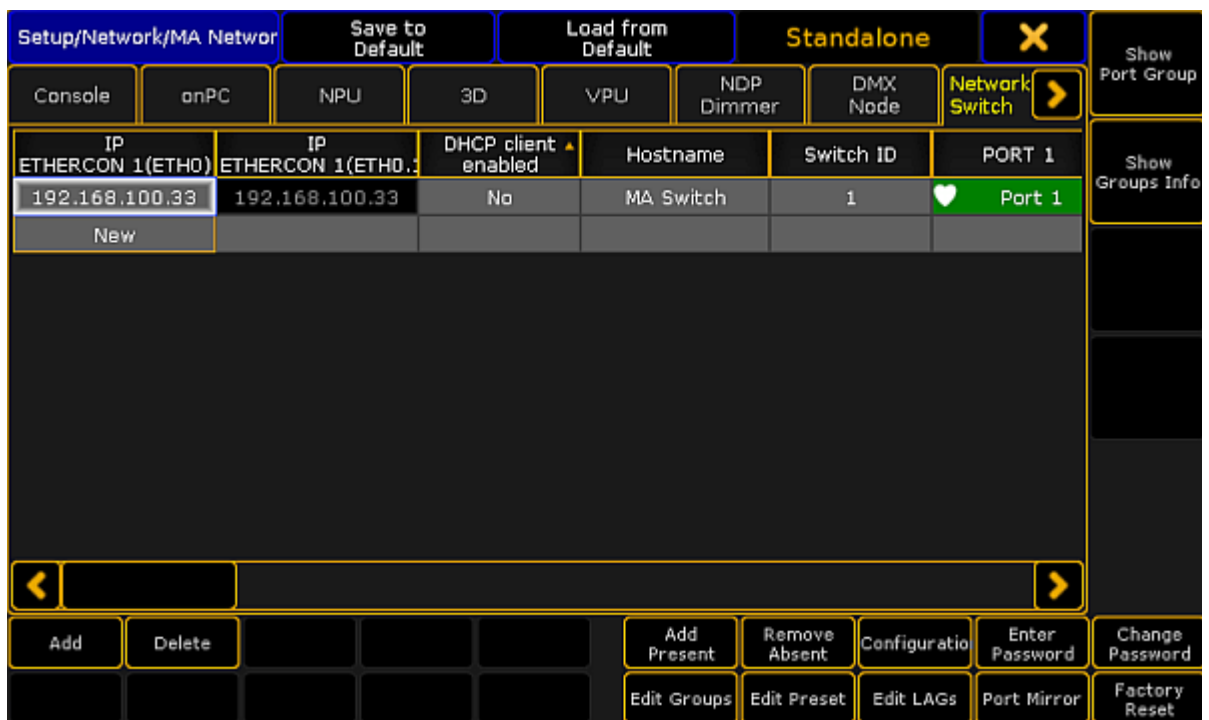
MA Network Configuration - Network Switch
